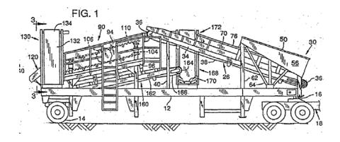
'564 patent fig.1. Material to be sorted is placed in the hopper 30. It is carried up by transport conveyor 26 and dropped onto screen assembly 90, which sifts it. Sorted material either descends down chute 120, or is carried away by conveyors 130 or 168, according to where in the sifting process the sorted material left the main stream.
